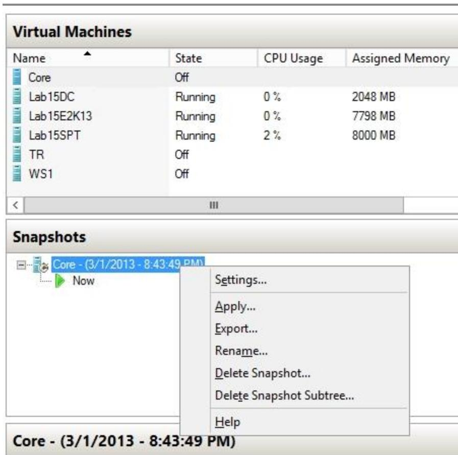
**Figure C:** You can rename a virtual machine’s previous state by right clicking on it and choosing the Rename option from the resulting shortcut menu.
